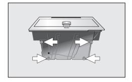
Push the machine all the way into the niche until there is a resistance. Then check the height to make sure it is sitting centrally in the unit and that it is level.
